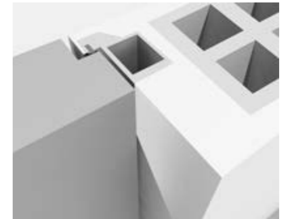
Porta filomuro lato interno, apertura a tirare Flush to wall door with inside pull opening
